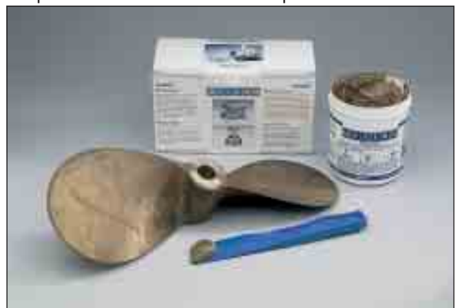
Picture 6 Repair of a ship's propeller
