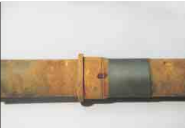
Picture 2 Repair of a primary shaft
