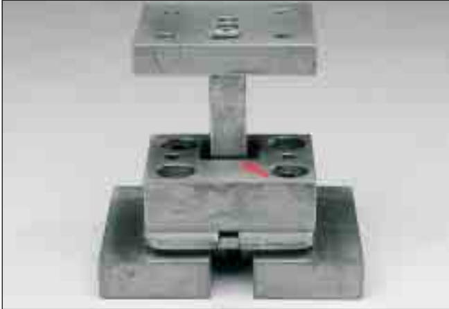
Picture 1 Repair of a guide in blancing press
