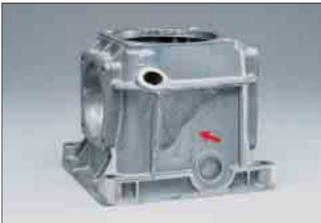
Picture 2 Reconditioning of aluminium housing
