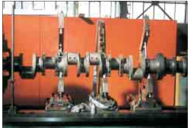
Picture 2 Crank shaft of a Diesel generator
