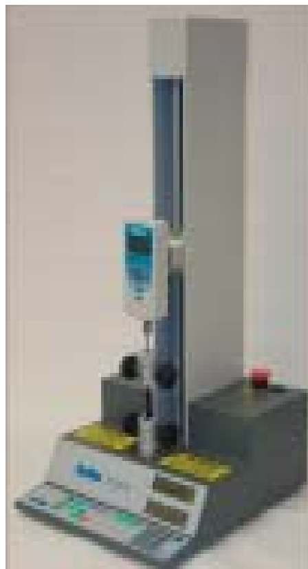
DFS Series force gauge shown with a TCD200 digital tester.
