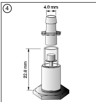
Gases can be inserted or withdrawn through the use of either sample line tubing or a syringe with a Luer-taper barrel fitting. This valve can eliminate the need to work with syringe-needles, if desired. The Luer-Fit Valve™ is also compatible with our full line of sampling accessories, including the Hann-Pump™.
