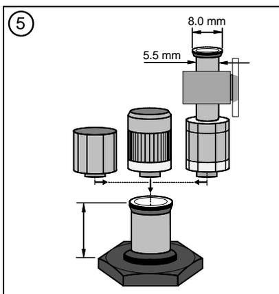
The Stopcock-Valve is one of our most popular valves because of its many different applications. This valve allows the user to control the flow of gas with greater flexibility. It consists of two pieces - a stopcock-base and a stopcock valve assembly which connects independently to the base by means of a rotating locking nut. (Figure left to right: Closing Cap "STOPCK-DE/1500", Stopcock-Septum "STOPCK-SEP", 1-way-Stopcock "STOPCK-ROT/L1200")
