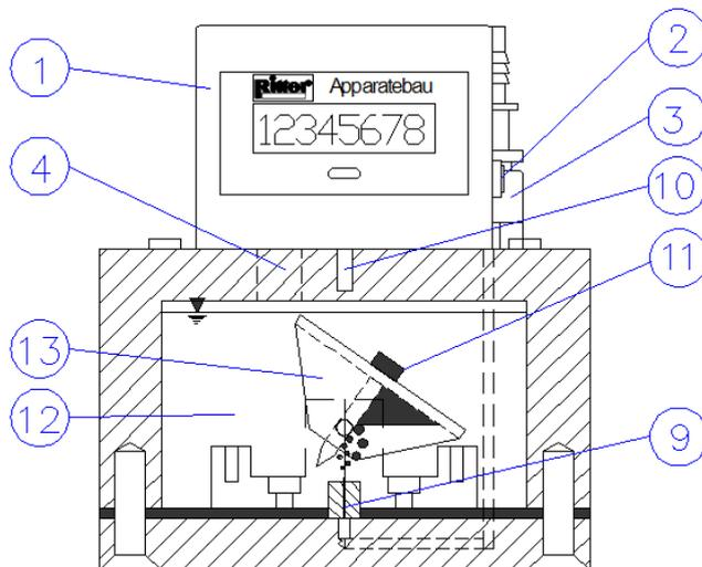
The gas to be measured flows in via the gas inlet nozzle (3), through the micro capillary tube (9) located at the base of the MilliGascounter and up into the liquid casing which is filled with a packing liquid (12).
