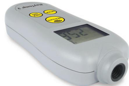
Designed and manufactured here in the UK, the new RayTemp 2 infrared non-contact thermometer is the latest addition to our range. Simply aim the thermometer at the target and press the measure button to display the surface temperature over the range of -49.9 to 349.9 °C with a 0.1 °C or 1 °C resolution and assured accuracy of  $\pm 1$  °C over the range 0 to 100 °C.
