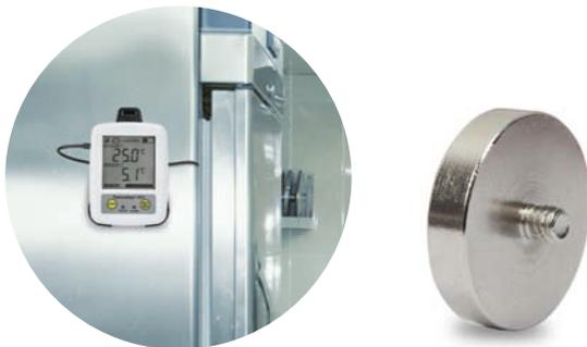
This new magnetic mount has been specifically designed to attach to wall bracket (832-590) and silicone boot (830-880) to allow for easy, convenient fixing to fridges, freezers and other ferrous metal surfaces. The magnet has a diameter of Ø36 mm with a thread size of 1/4-20 UNC.
